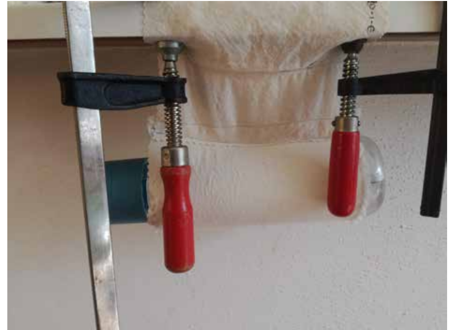
Figure 40. Setup for the strength test of a fold
