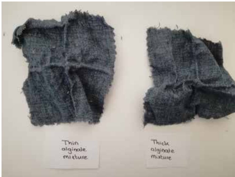
Figure 25. Linen fabric with 3(left) and 5 (right) w/v% alginate
