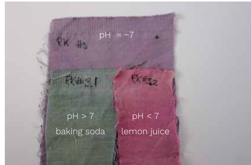
Figure 1. Effect of pH on red cabbage dye
